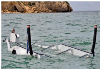
Both trailers floating at anchor, Bill's with additional buoyancy provided by a bladder system he can inflate with an electric pump, plus aluminium 'wings' over the guide poles
