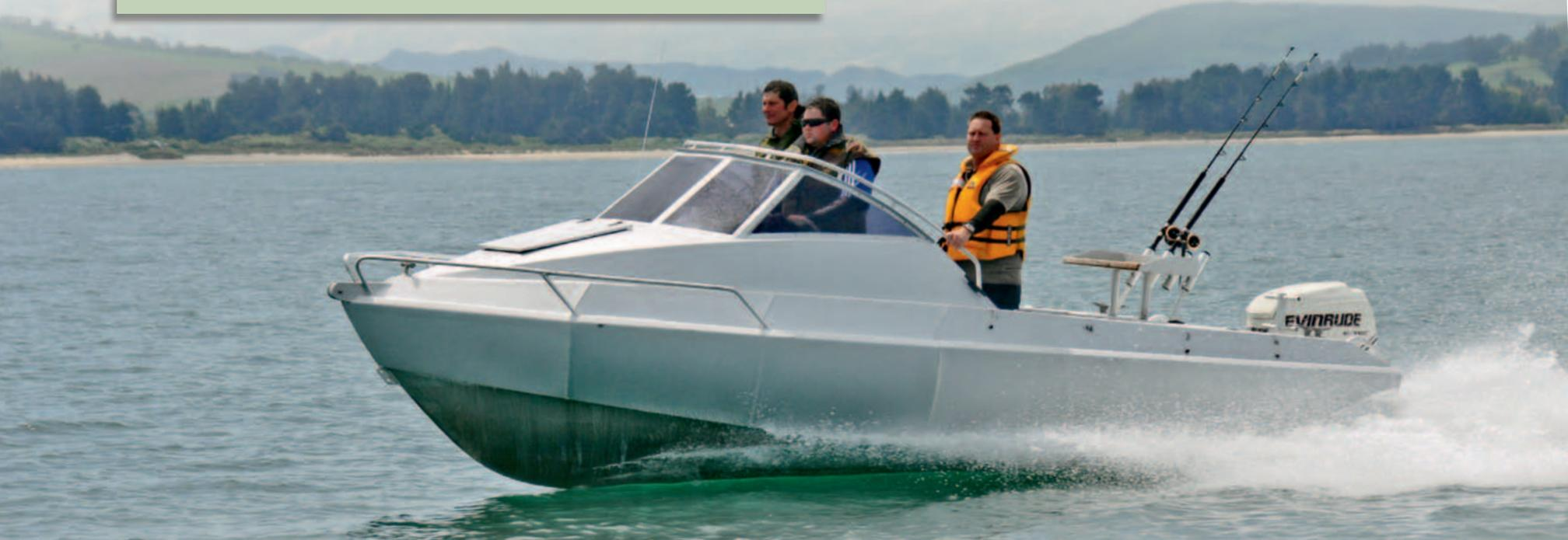
**Revo Beachcraft 601 Pontoon** ▶ loa 6m ▶ beam 2.389m ▶ Internal beam (cockpit) 1.755m ▶ draft approx 300mm, motor up ▶ weight approx 1000kg (wet, plus trailer) ▶ engine 130-150hp outboard ▶ deadrise variable to 18.5° at transom ▶ fuel 100-litre underfloor tank ▶ price as reviewed \$67,000 including trailer (Nathan's boat) ▶ enquiries Beachcraft Boats Ltd, 021 972578 or 09 5308374, boats@revo.co.nz or www.revo.co.nz
